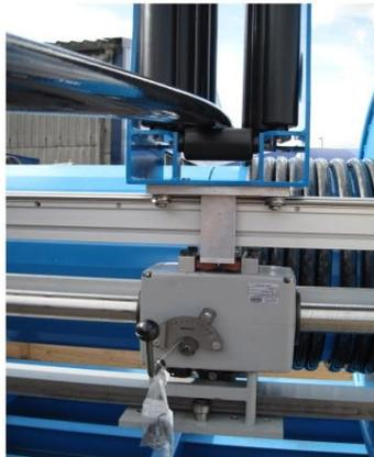
*Uhing ARG4-60 Rolling Ring Drive/ Assembly with Load Carrier
