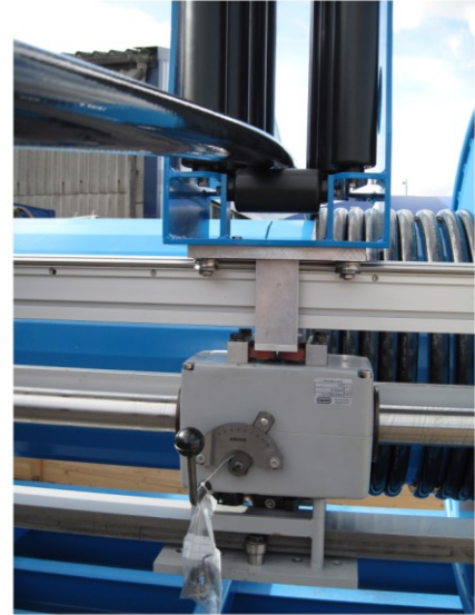
Uhing ARG4-60 Rolling Ring Drive/ Assembly with Load Carrier Photo: Keith Makinson, BAS
