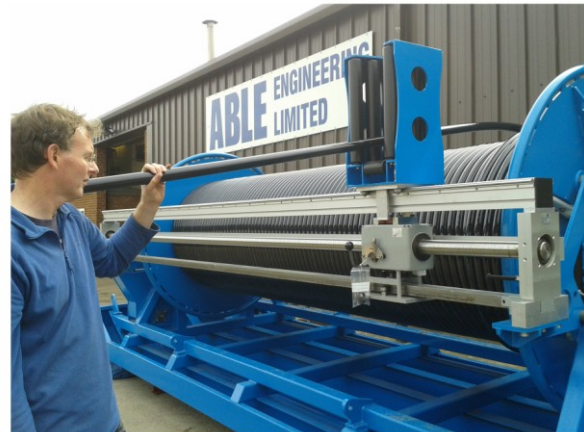
The BAS custom winding machine, Photo: Emily Venables, BAS
