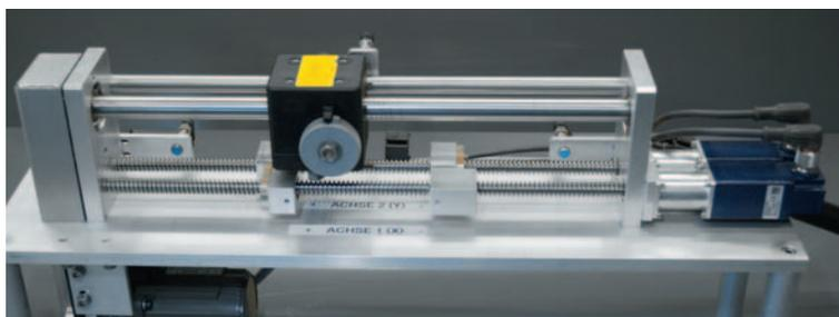
Corrections are possible with the handwheel during operation.
