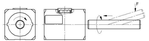
Turn anti-clockwise for a drive nut with a left-hand rolling direction
